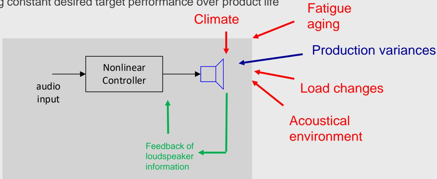
An adaptive, nonlinear control system is required !
