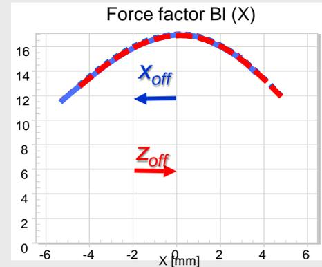
Force factor  $BI(x)$  versus absolute voice coil position referenced to gap geometry
