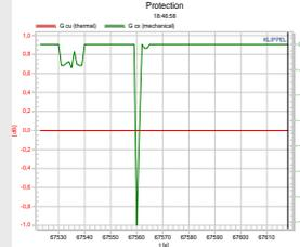
Activation of mechanical and thermal protection
