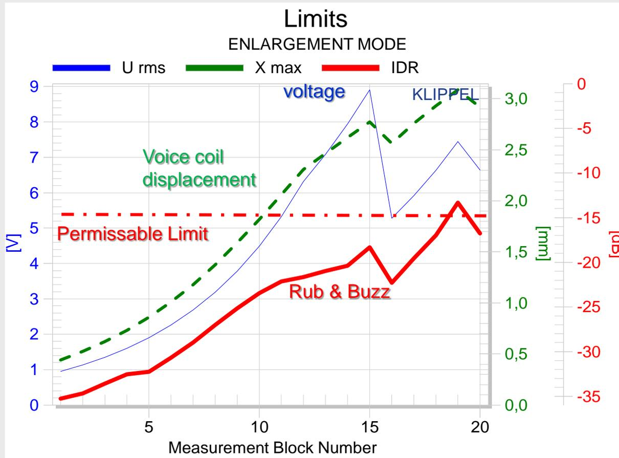
The measurement of impulsive distortion is the most important criteria to find the limit of the operation range
