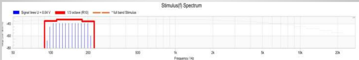
Low frequency band generates the voice coil displacement that activates the loudspeaker nonlinearities
