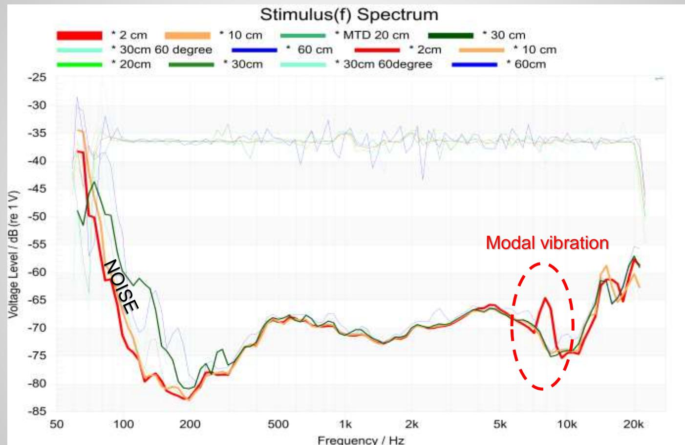
Equivalent input MTD are almost independent of the microphone position
