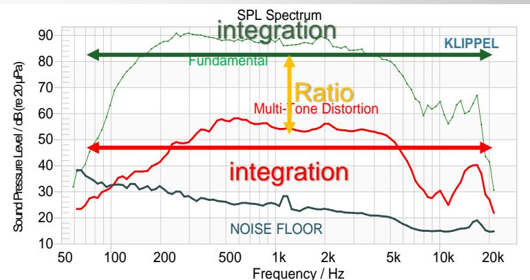
$$R_{\text{SMTD}}(f_i) = 10 \lg \left( \frac{\int_{f_{i-1}}^{f_{i+1}} |P_{MD}(f, \mathbf{r}_{\text{near}})|^2 df}{2 |P(f_i, \mathbf{r}_{\text{near}})|^2} \right) \text{dB} \quad i = 2, \dots, N-1$$
