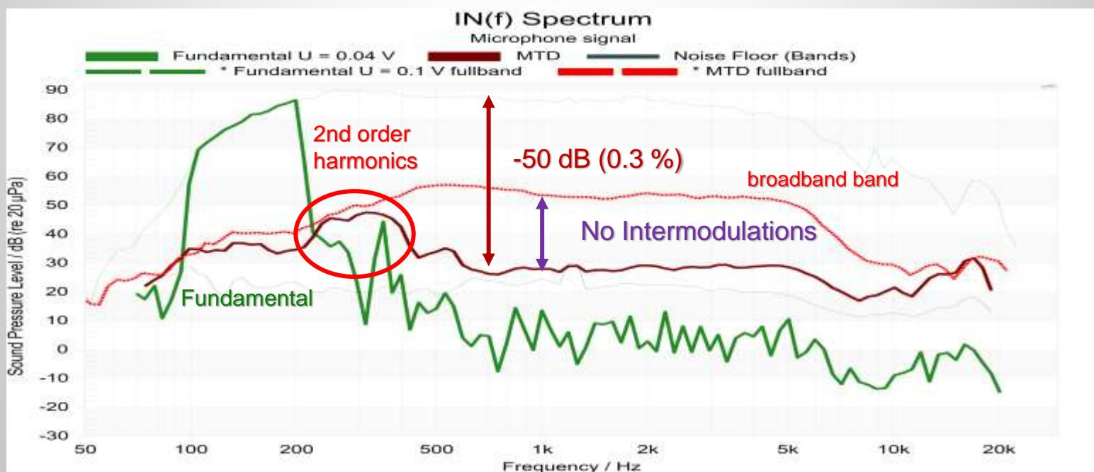
The intermodulation generates 20 dB more distortion in the audio band !!
